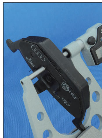
测量刹车片槽深
